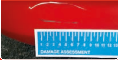
Bumper scratch over 25mm
