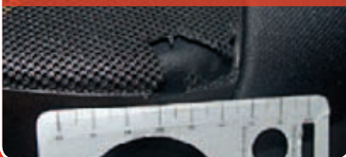
Speaker mesh damage
