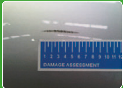
Scuff on surface not penetrating base material
