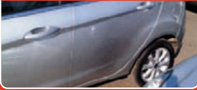
Poor repair: repainted panel does not match
